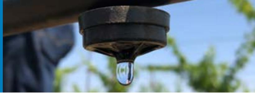
**Flushing the main, sub-main and distribution lines will considerably reduce the accumulation of organic and mineral materials in the system. This will help prevent those materials from reaching the drippers and eventually clogging them.**
